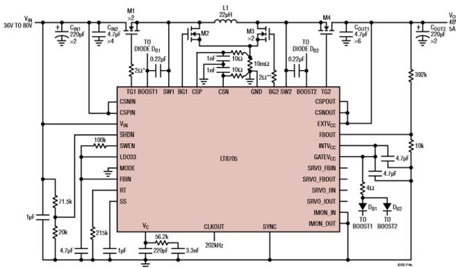
**Figure 7: Typical layout of LT8705 configured for variable input with fixed output**
