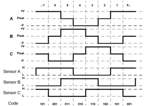
**Figure 4: Sensor vs Drive Timing**
