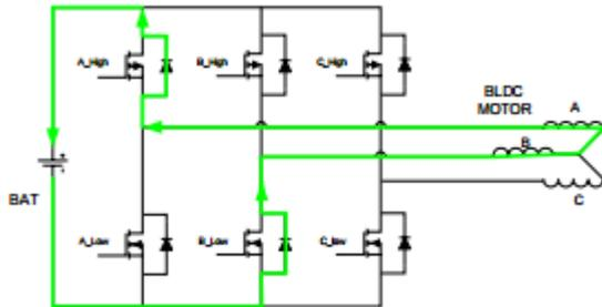
**Figure 5: Regenerative Braking Current**
