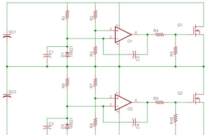
**Figure 8: Schematic of the charge limiting circuit.**
