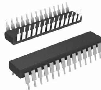
**Figure 6: PIC16F886 microprocessor**
