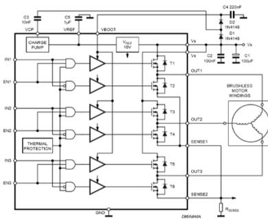
**Figure 2: L6234 Block Diagram**
