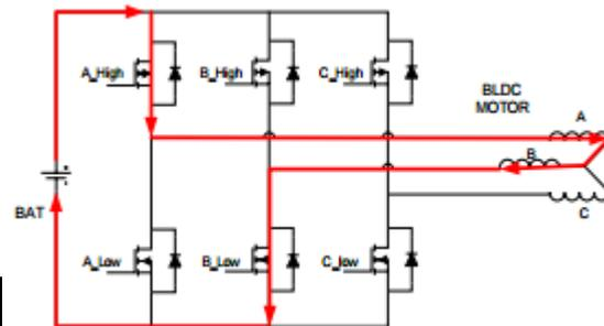
**Figure 3: Motor Current Flowing**
